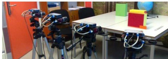
Figure 1: Four stereo cameras capturing a scene.
