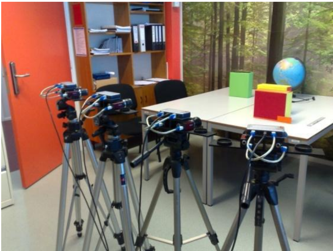
Figure 5 – Ordinary stereo camera setup with four stereo cameras positioned around a scene.
