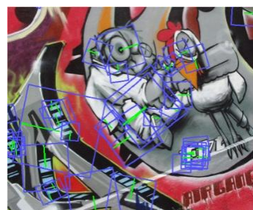
Figure 34 – Visualization of interest point scale and orientation as found by SURF
